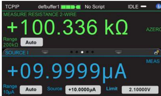
Figure 70: Resistance measurement with automatic settings
