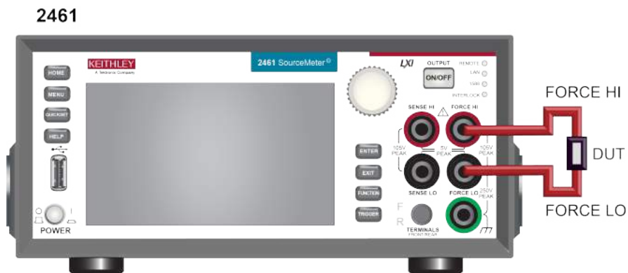
Figure 59: 2461 2-wire rear-panel connections
