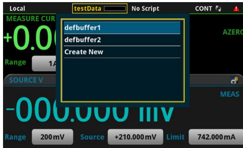
Figure 184: 2461 active buffer indicator expanded
