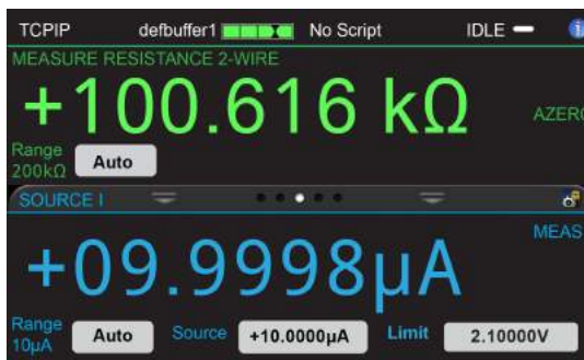
Figure 69: Resistance measurement using resistance function
