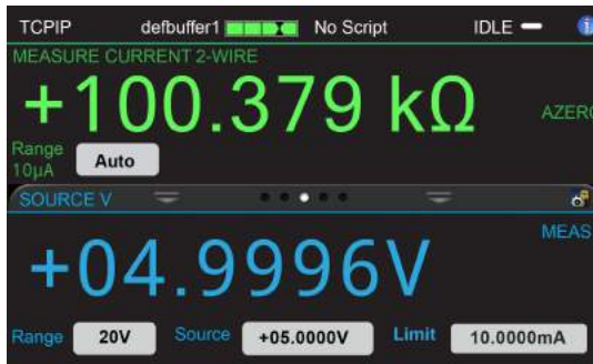
Figure 66: Resistance measurement SVMI and reading ohms
