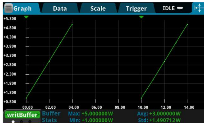
Figure 135: Graph with data from a writable buffer with start group markers
