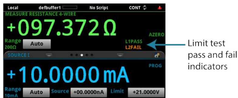
Figure 96: Limit test front-panel indicators
