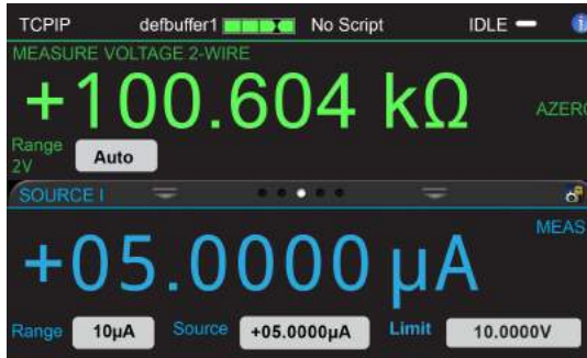
Figure 67: Resistance measurement SIMV SCPI example
