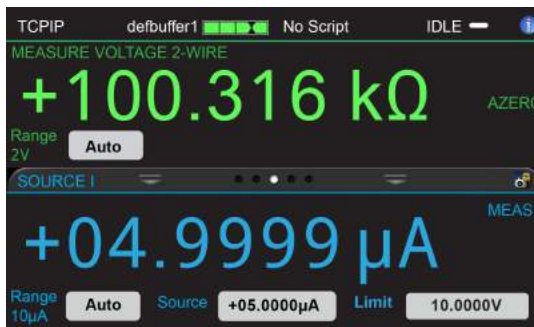
Figure 68: Resistance measurement SIMV and read ohms
