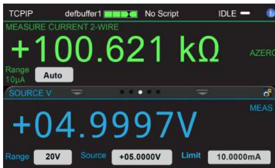
Figure 65: Resistance measurement using SVM1 and reading ohms
