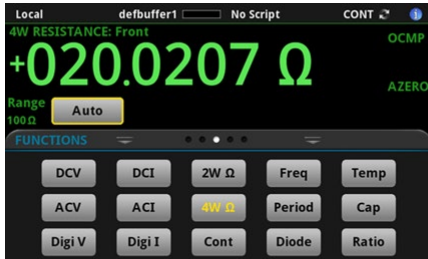
Figure 37: 4-wire resistance test results
