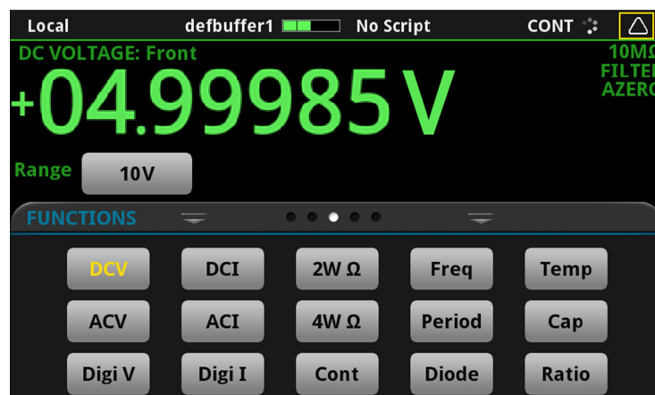
Figure 34: DC voltage high-accuracy test results
