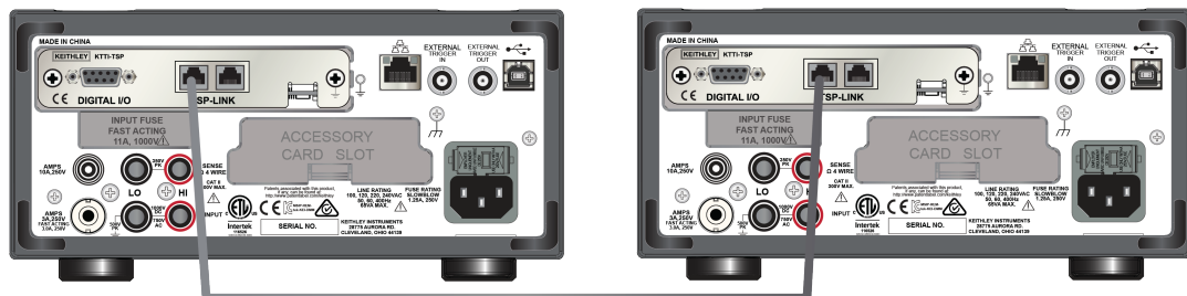
Figure 43: Two DMMs connected with TSP-Link
