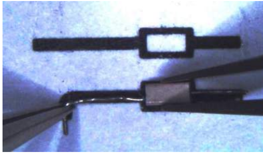
Figure 97 Resistor Placed on the Bend Detail Outline
