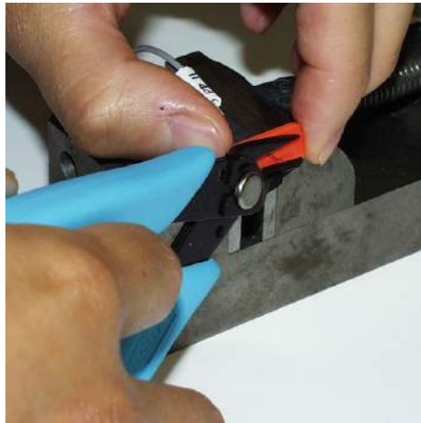
Figure 93 Cutting Wires Flush with Gauge
