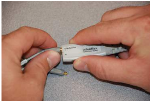
Figure 4 Properly Pulling the Probe Head Straight Out
