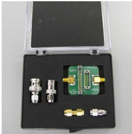
Figure 113 N2887-60002 Calibration/Deskew kit
