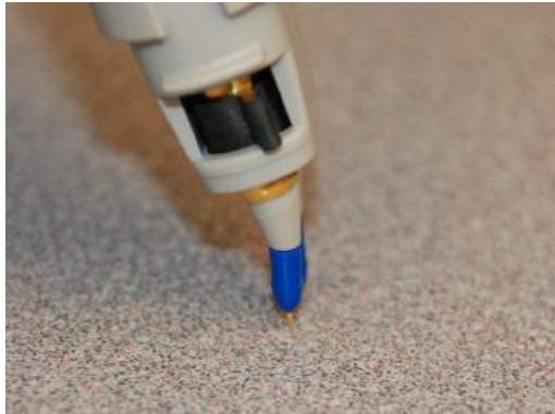
Figure 55 Proper Vertical Orientation of the Blue Tips
