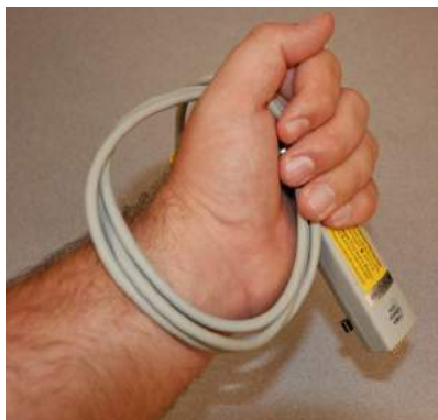
Figure 6 Recommended Coil for Storage
