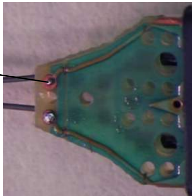
Figure 91 Wire Cut Flush with Solder pad
