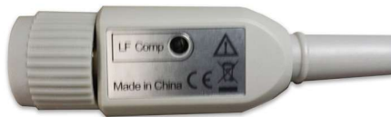
Figure 2. Low-frequency compensation adjustment (for N2840A/41A/42A/43A/53A)
