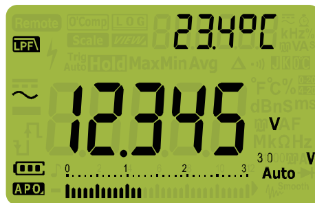
Figure 2-3 AC voltage with LPF display
