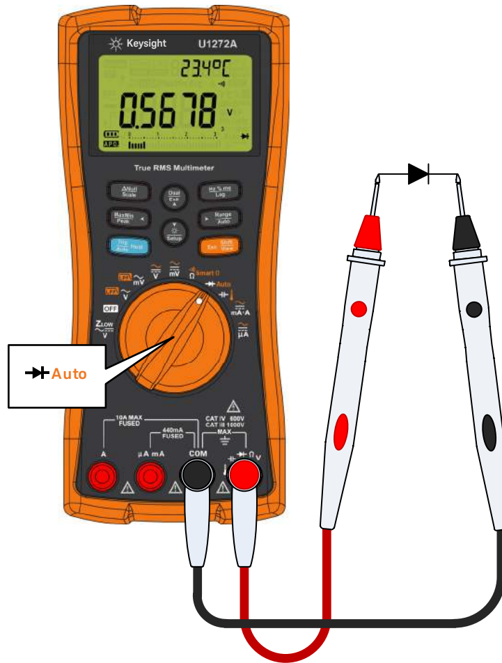
Figure 2-21 Testing forward bias diode
