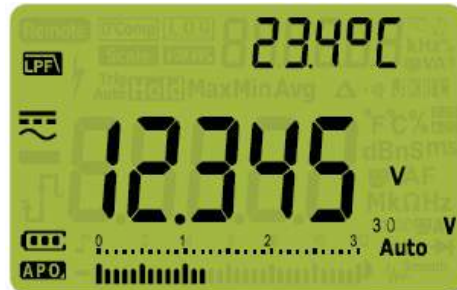
Figure 2-8 Low Pass Filter(LPF) for AC+DC voltage measurements
