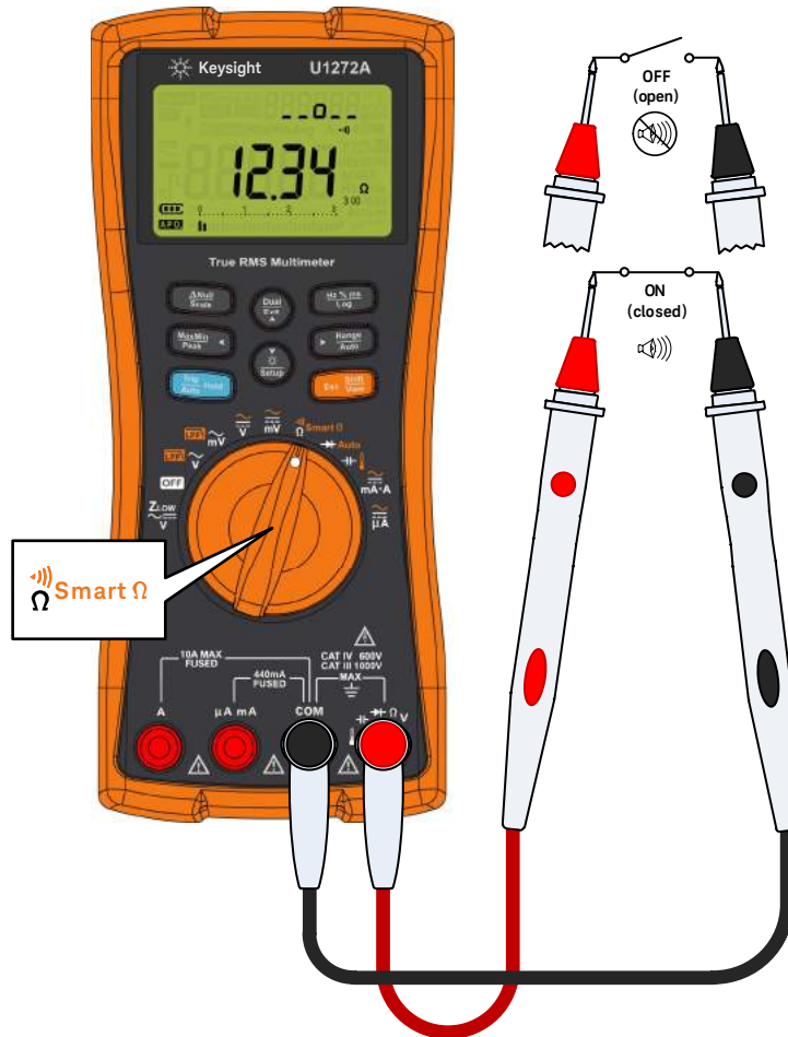
Figure 2-16 Tests de continuité
