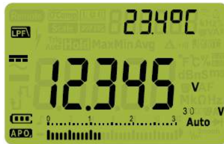
Figure 2-6 Filter for DC voltage measurements
