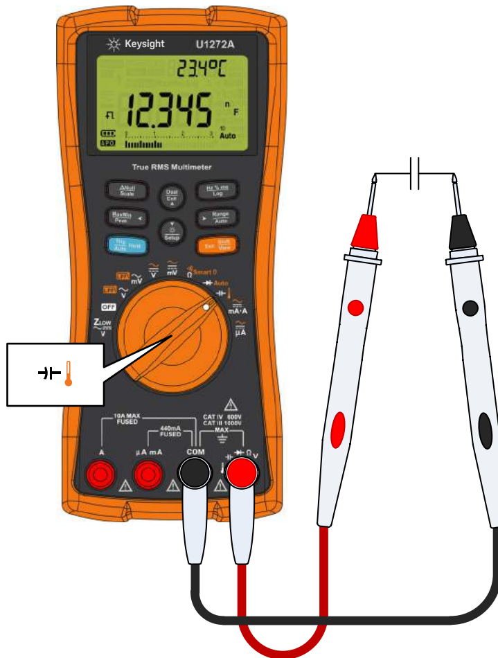
Figure 2-26 Measuring capacitance
