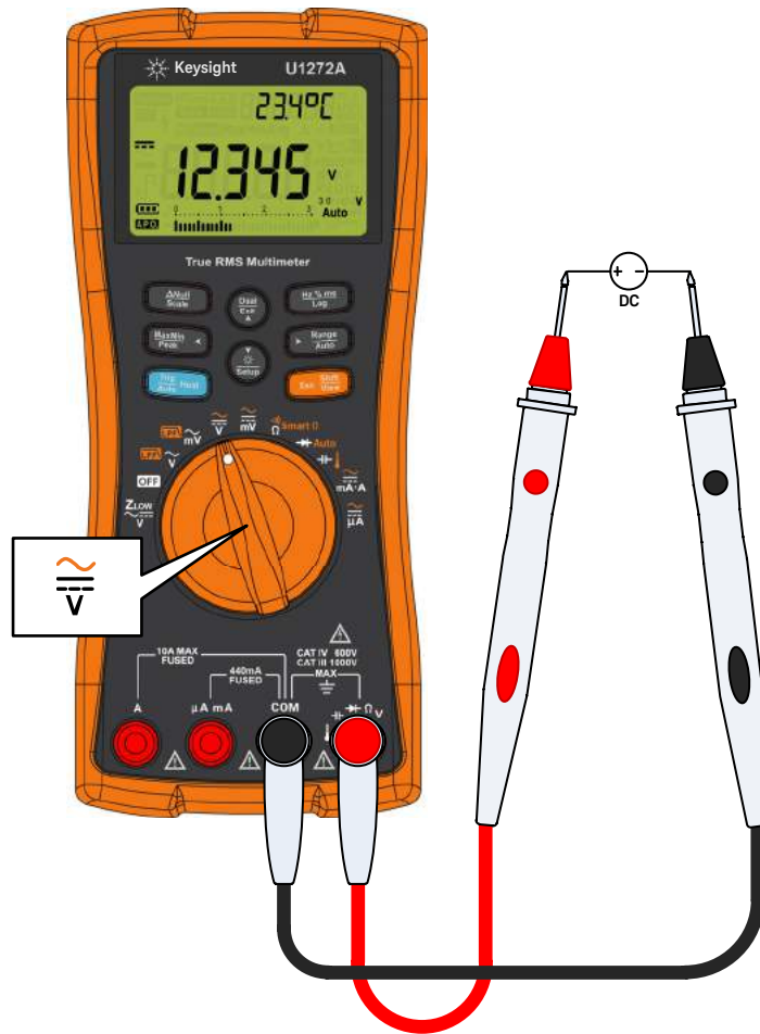
Figure 2-5 Measuring DC voltage
