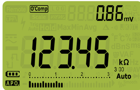
Figure 2-17 Smart \Omega (with bias voltage) display
