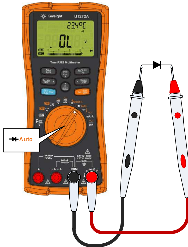
Figure 2-22 Testing reverse bias diode
