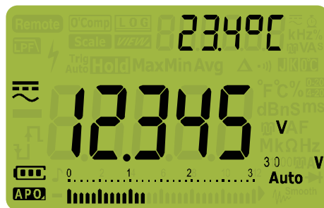
Figure 2-7 AC+DC voltage display
