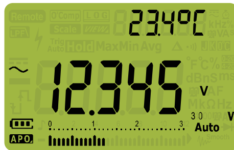
Figure 2-1 AC voltage display
