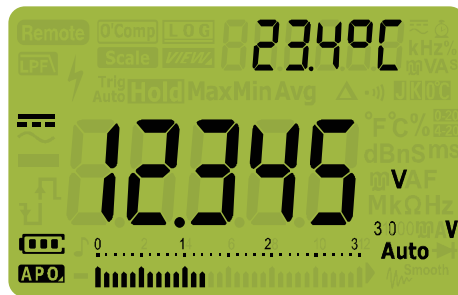
Figure 2-4 DC voltage display
