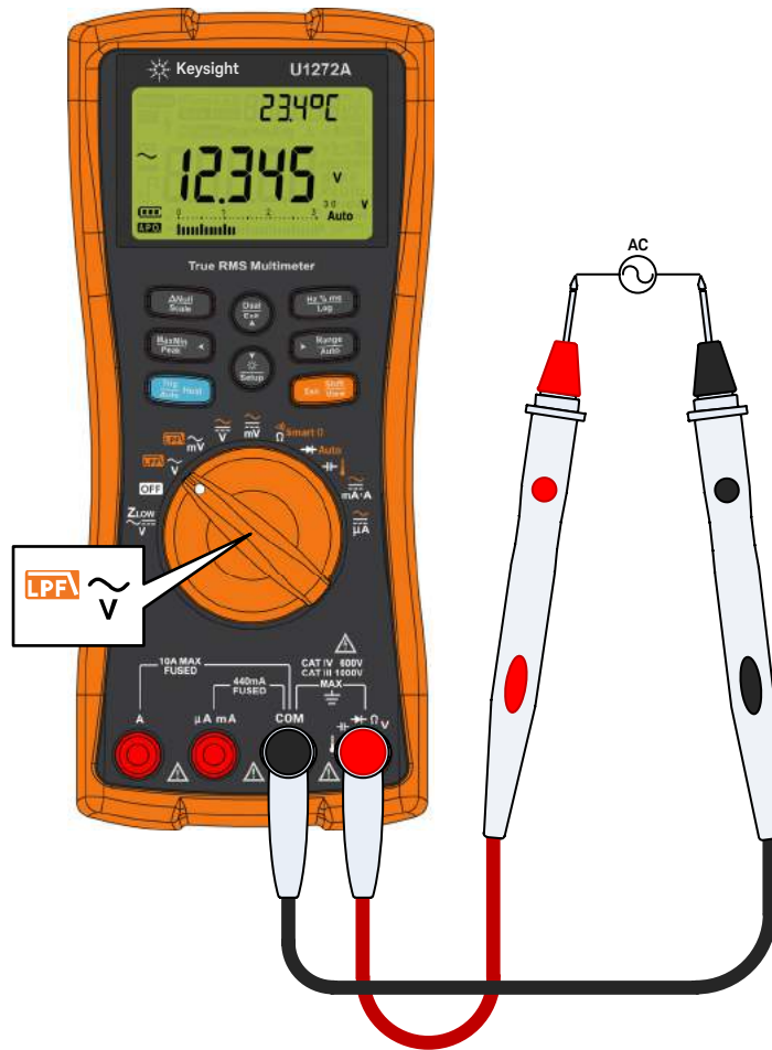
Figure 2-2 Measuring AC voltage
