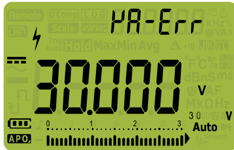
Figure 1-3 Input warning display
