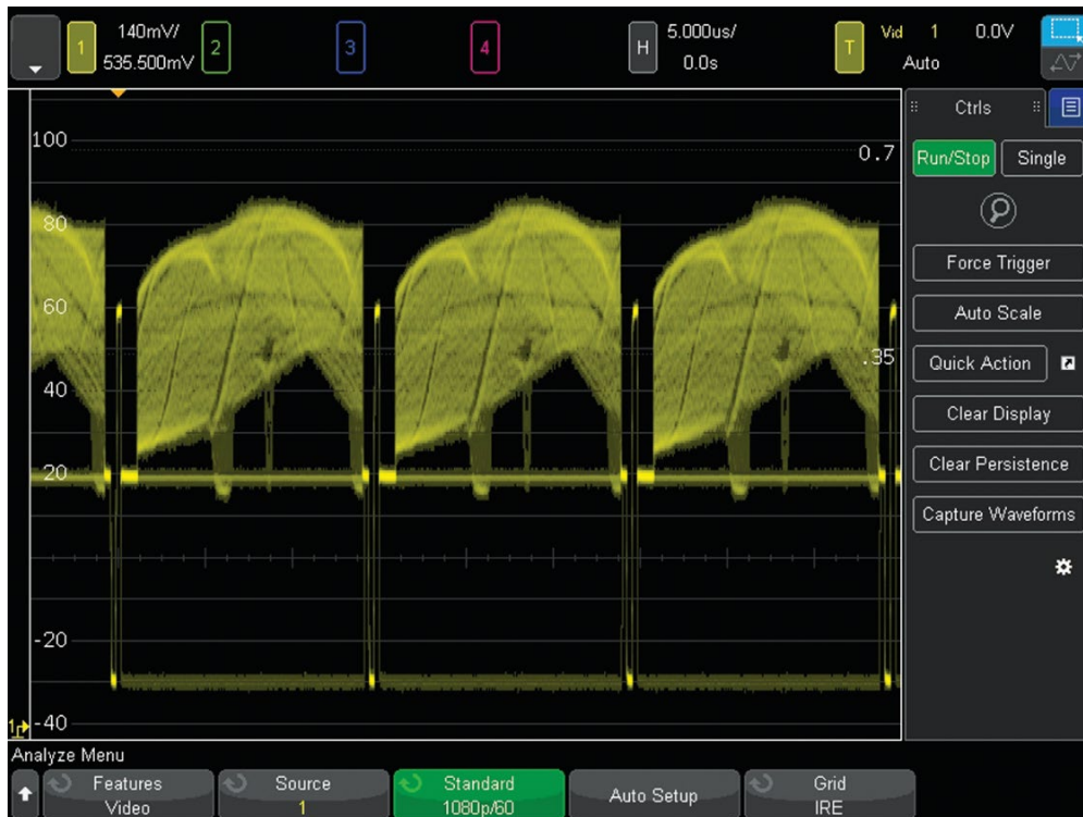
Figure 9. Triggering on 1080p HDTV.
