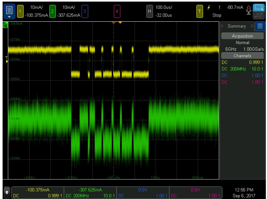
Improved noise floor of the N7026A (yellow trace) over the N2893A (green trace)
