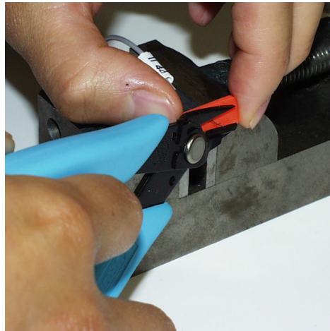
Figure 93 Cutting Wires Flush with Gauge
