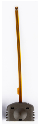
Discoloration after usage under high temperatures
