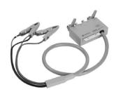
Terminal connector: 4-Terminal Pair, BNC DUT connection: 4-Terminal
