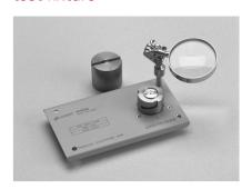
Terminal connector: 7 mm DUT connection: 2-Terminal Electrical length: 26.9 mm Dimensions (approx.): 140 (W) x 48 (H) x 78 (D) [mm]
