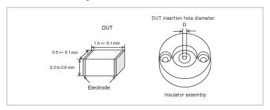
The 16196B is furnished with three different insulator assemblies, since any gaps between the DUT and the cylindrical insulator will result in improper positioning and subsequent measurement errors. Select an insulator assembly that reduces the gap the most. See the table below for dimensions of the insulator assemblies.
