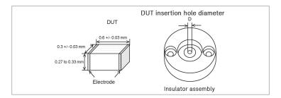
The 16196C is furnished with one insulator assembly. See the table below for the dimensions of the insulator assembly.
