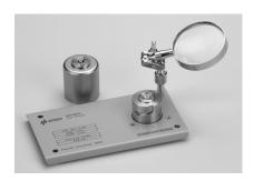
Terminal connector: 7 mm DUt connection: 2-Terminal Electrical length: 27.3 mm Dimensions (approx.):
