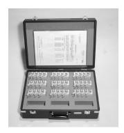
Terminal connector: 4-Terminal pair, BNC Dimensions (approx.): 94 (W) x 31 (H) x 67 (D) [mm] (resistors) Weight (approx.): 3.7 kg (including case and 9 resistors)
