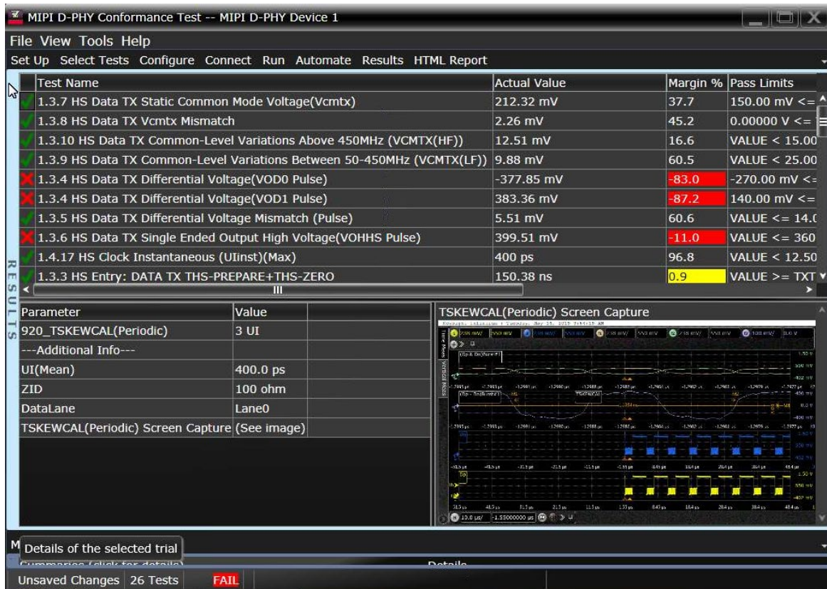
Figure 3. Results reports quickly highlight test margins versus specified limits and a summary of measurements that pass/fail or violate the margin warnings you have set.
