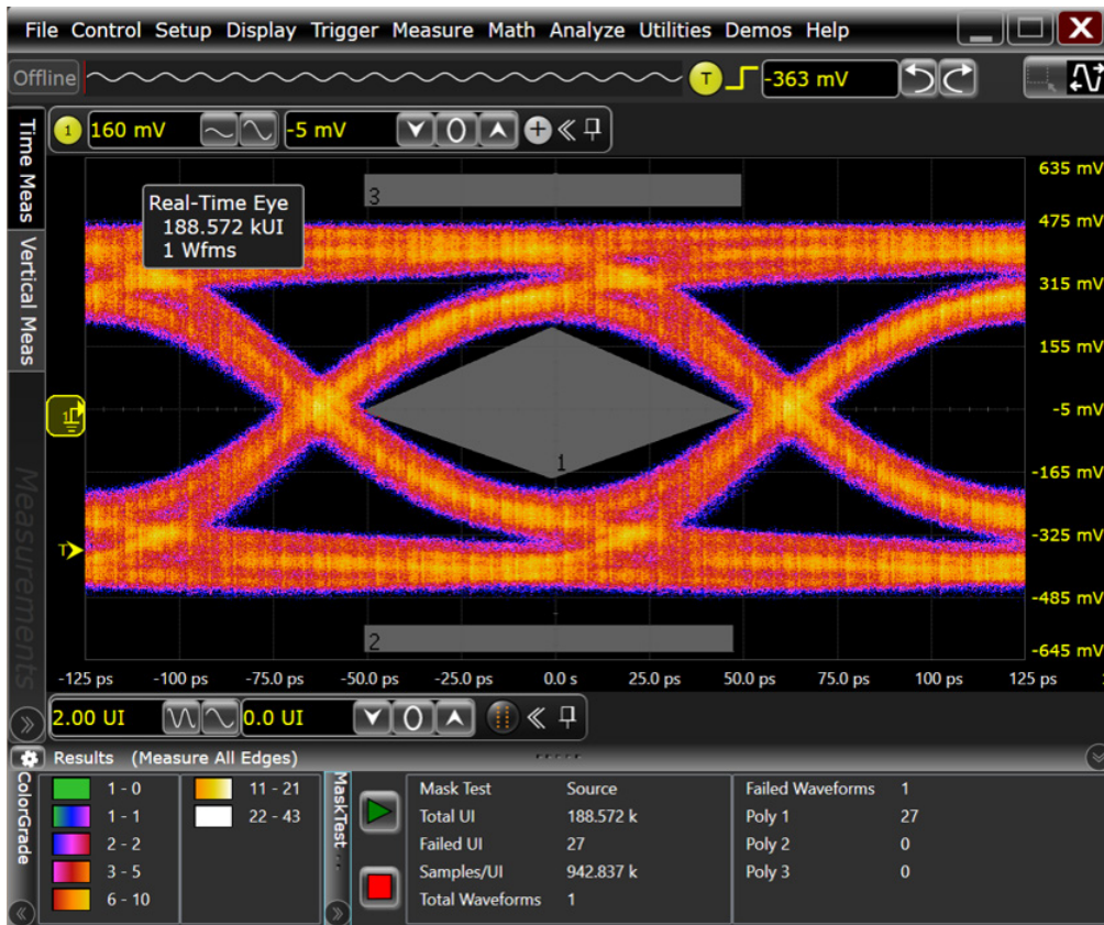
Figure 21. The Serial Data Analysis and optional D9020ASIA Equalization applications allow for the equalization of impaired 8 and 16 Gb/s signals so a clock can be recovered and mask testing can be performed on your waveforms
