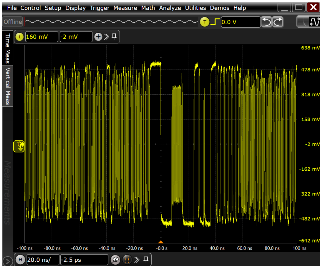
Figure 1. PCI Express 4.0 supports data rates up to 16 GT/s as shown above (P4 preset)
