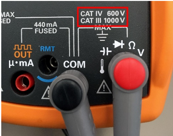
Figure 1. Digital multimeter with IEC measurement category highlighted within the red box.
