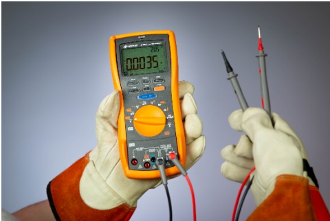
Figure 2. Using insulated gloves to make live measurements.
