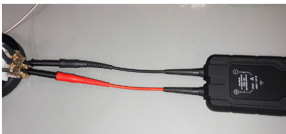
Figure 6 DP0001A Input leads running in parallel (Best case)
