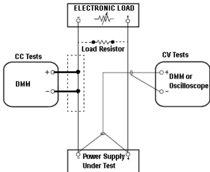
This setup is used for most tests and it requires the DMM, electronic load, and power supply being verified. Some wire is also required for connection between instruments. A LAN or USB cable is needed for readback data. The
