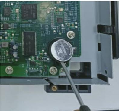
4. Install the new battery. Make sure that the positive side (+) is facing up. Place the battery under the small spring (see red circle below) and push down on the opposite end of the battery (see red arrow below) to seat the battery.
