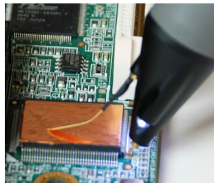
Figure 6 Copper Pad on IC
