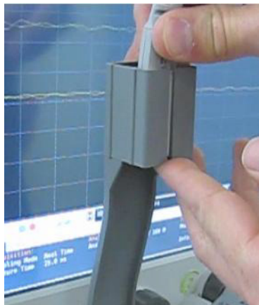
Figure 77 Inserting the Probe Head
