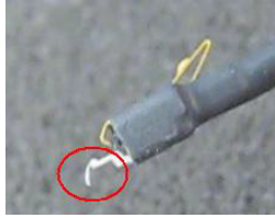
Figure 78 Forming the Probe Head's Tip
