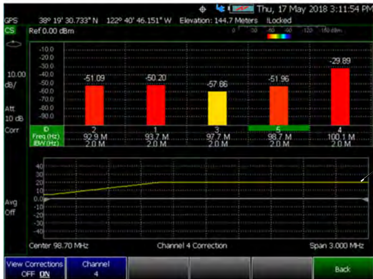
Figure 27-17 Yellow Trace with Cable and Antenna Corrections
