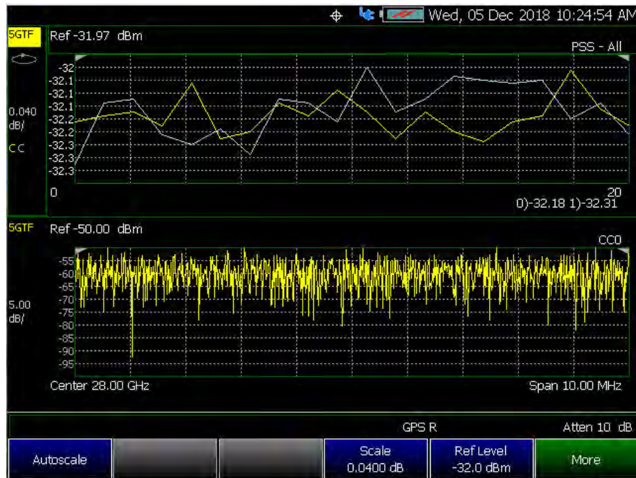
Figure 13-15 Spectrum and Strip Chart Display Type – 5GTF
