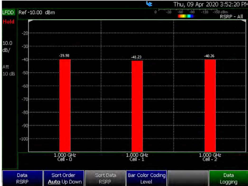
Figure 13-4 LTE FDD Bar Chart – Level Example
