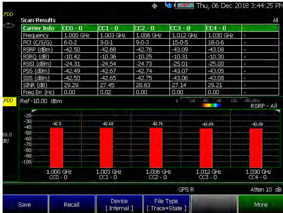
Figure 13-11 Example of LTE FDD with Multiple Carriers, Single Cell Site, and KPI's
