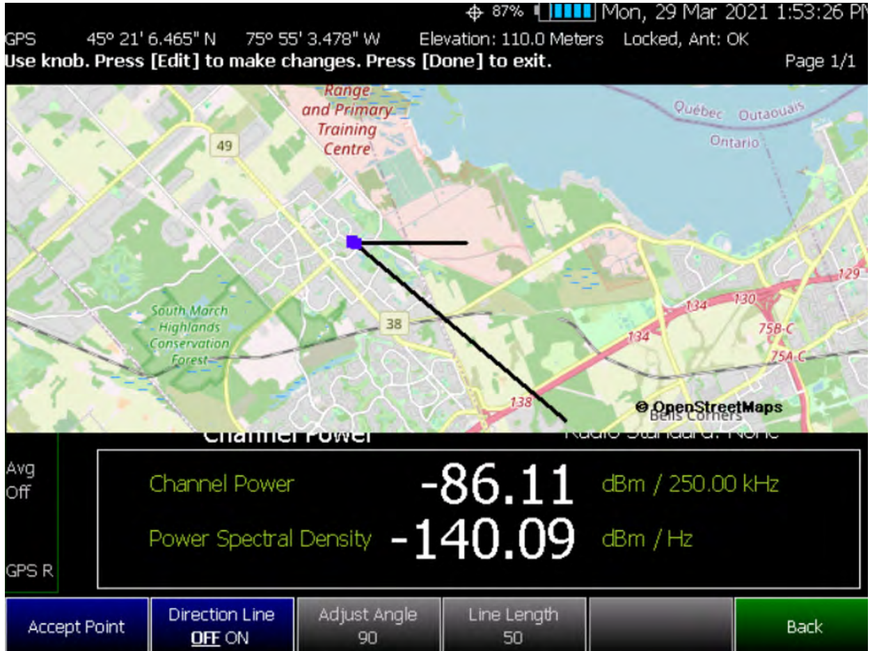
Figure 16-23 Directional Finding (DF) Bearing – Outdoor Map Data Logging Example
