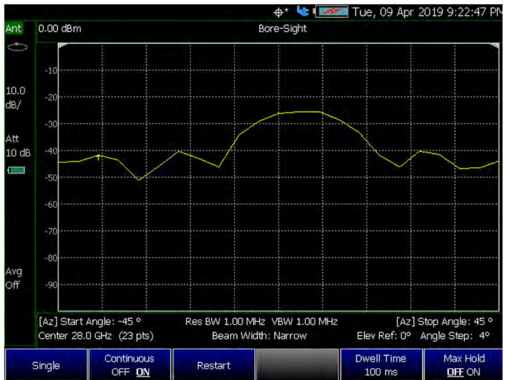
Figure 14-10 Bore-Site Measurement with Pulsed RF (Dwell Time=100 ms, Max Hold=OFF)
