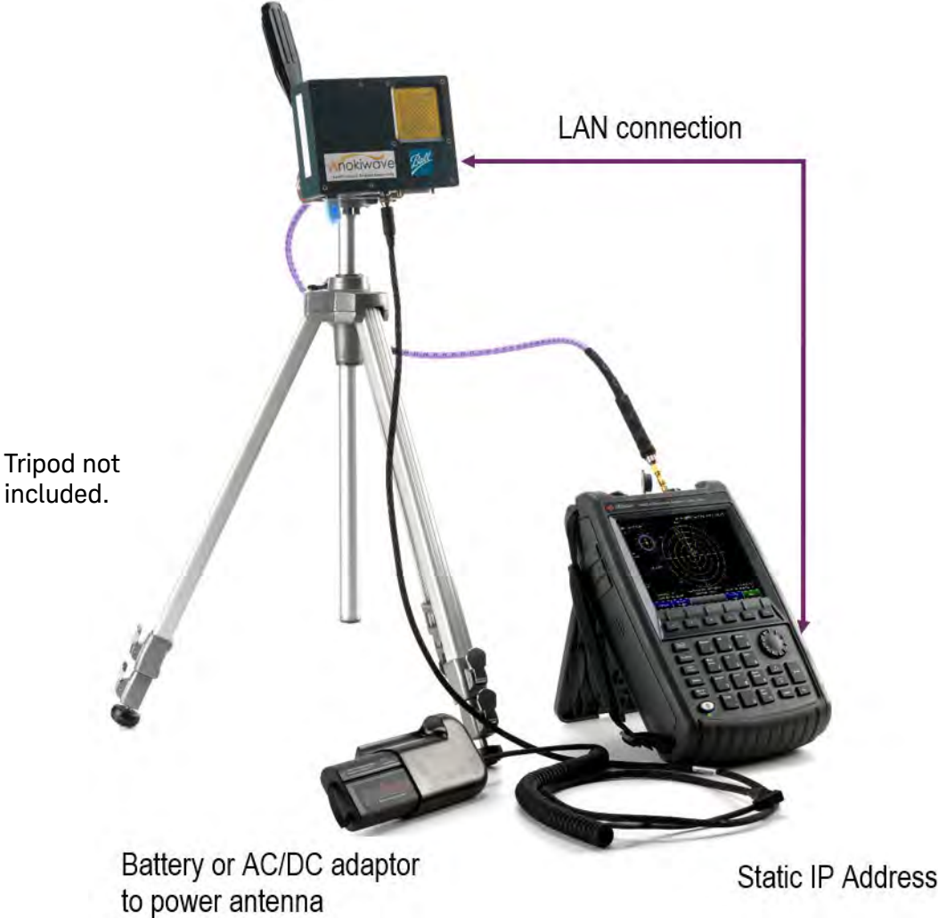
Figure 14-1 Example of local point-to-point LAN connection
