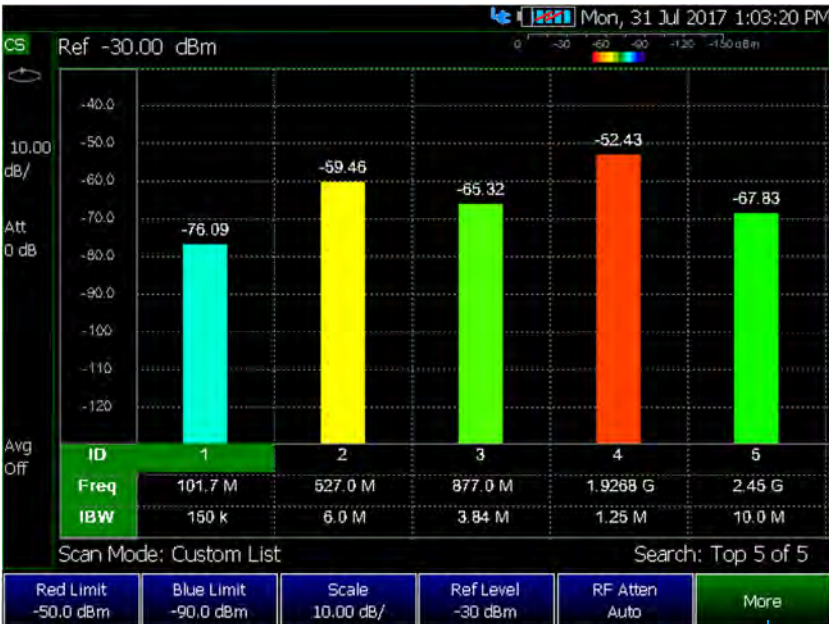
Figure 27-15 Overview of Field Strength for Channel Scanner (See also, Figure 27-16 on page 641 .)
