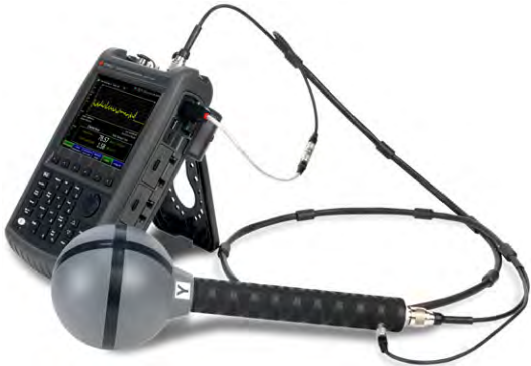
FieldFox With USB Antenna
