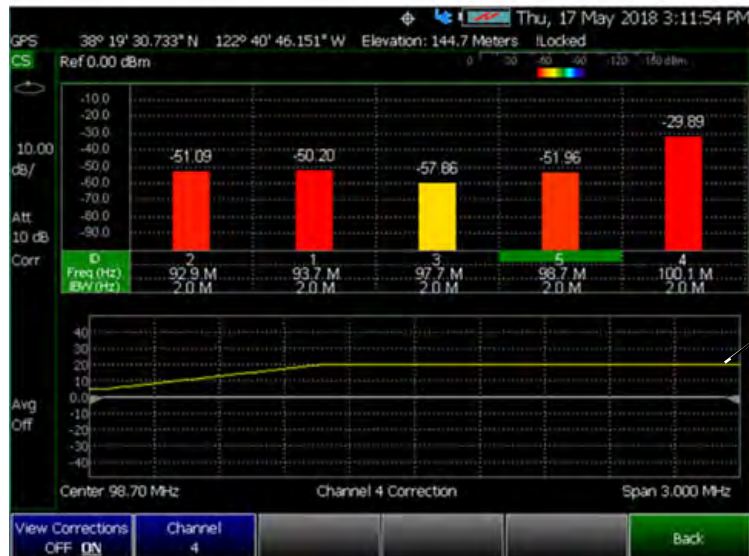
Figure 27-17 Yellow Trace with Cable and Antenna Corrections
