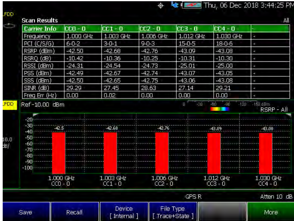
Figure 13-17 Example of LTE FDD with Multiple Carriers, Single Cell Site, and KPI's
