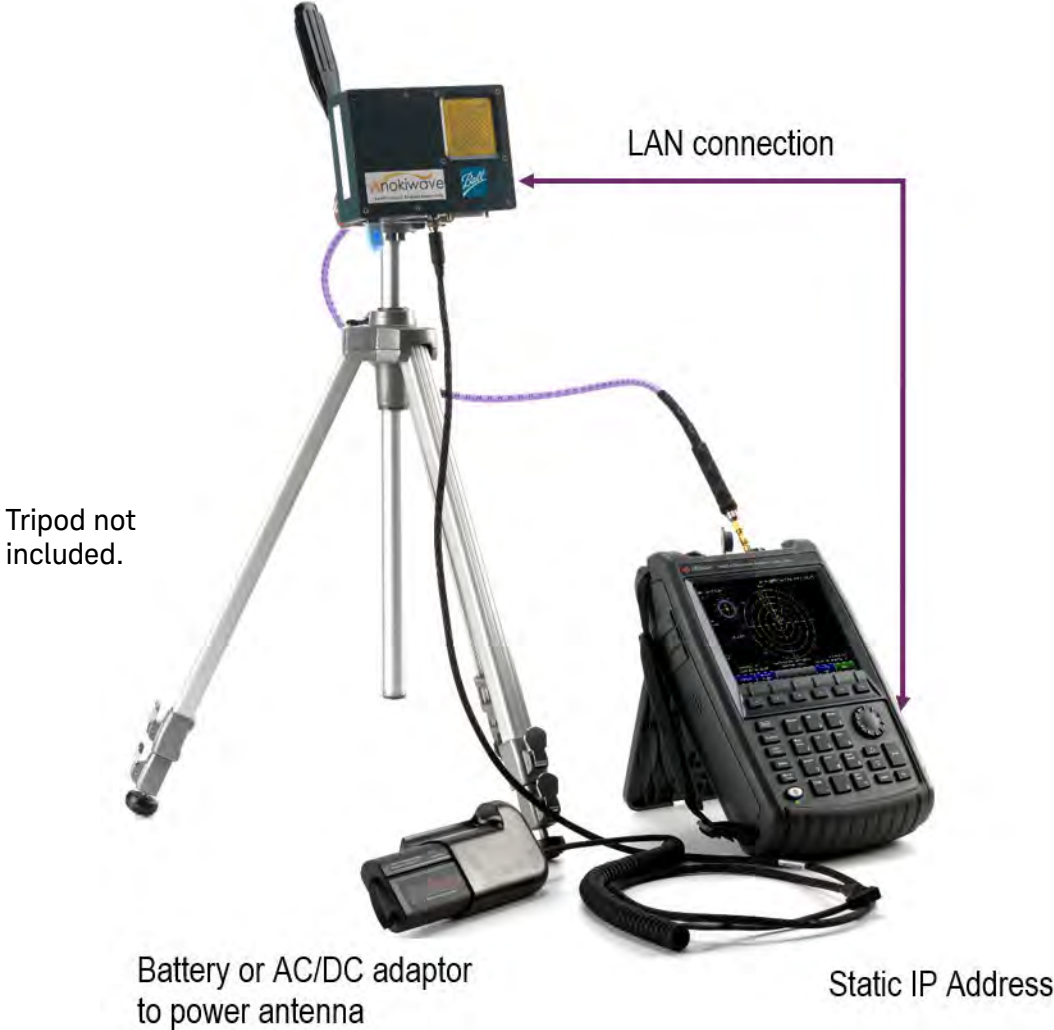
Figure 14-1 Example of local point-to-point LAN connection
