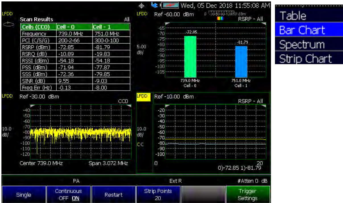
Figure 13-1 Example of the LTE FDD with Four Multiple Display Options – (LTE TDD is similar)
