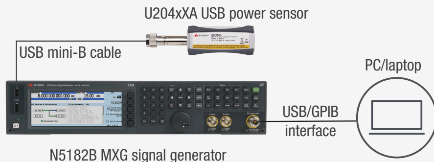
Figure 24. Connection diagram showing a USB power sensor connected to the N5182B MXG signal generator's USB port
