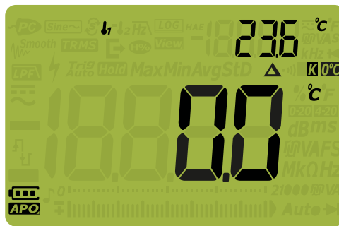
Figure 2-22 Temperature measurement without ambient compensation
