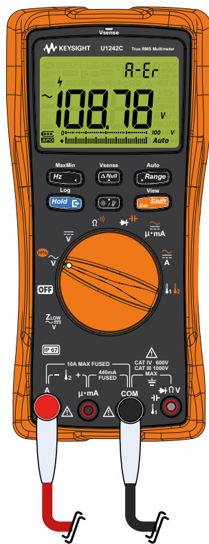
Figure 1-2 Example of wrong terminal input
