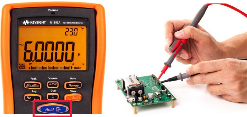
Figure 5. Hold & Export button—one press for three actions: Measure, save it into handheld DMM's memory and send the measurement out via infrared port. Optional U5404A remote switch probe emulates 'Hold & Export' button.
