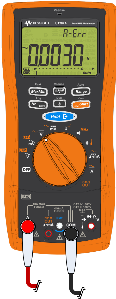
Figure 1-2 Example of A-Err for wrong terminal input
