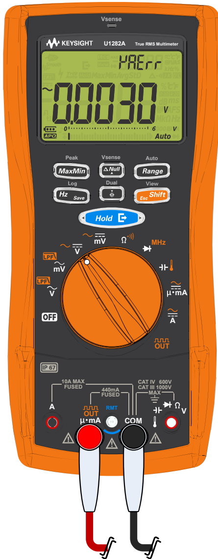
Figure 1-3 Example of \mu\text{AErr} for wrong terminal input
