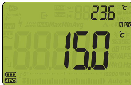
Figure 2-25 Temperature measurement without ambient compensation
