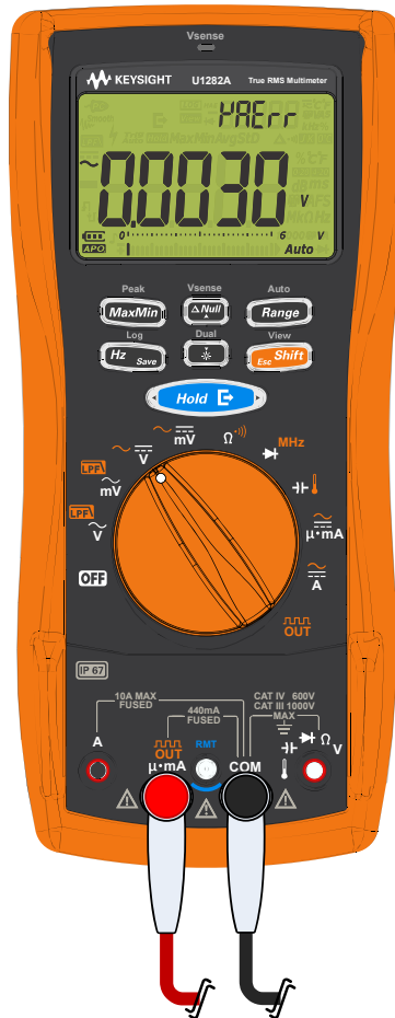
Figure 1-4 Example of wrong terminal input
