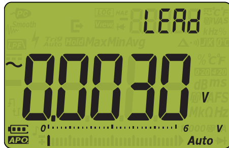
Figure 1-5 Input warning display
