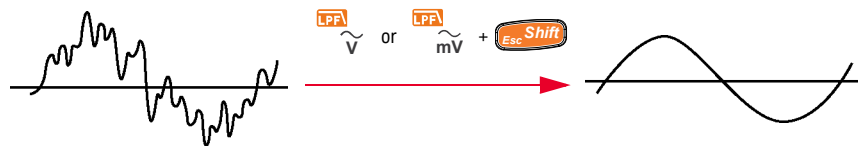
Figure 2-4 Low-pass filter operation
