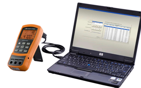
PC data logging with optional IR-to-USB cable.
