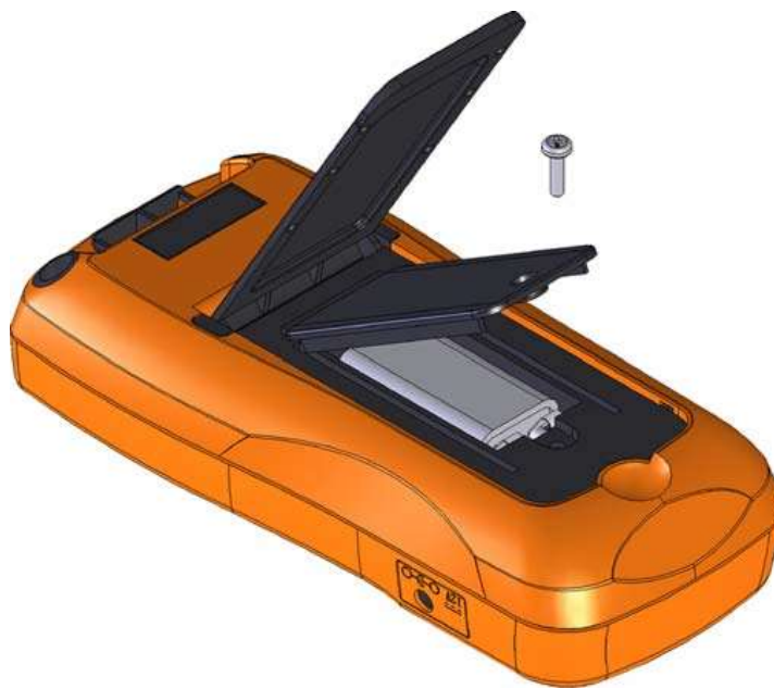
Figure 1-1 Installing the batteries
