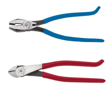
The Ironworker's Kit is a 2-Piece Pliers set that includes a heavy-duty side-cutter and angled-head diagonal cutter, both used to cut soft annealed rebar tie wire. The side-cutters (Cat. No. D2000-7CST) twist tie wire and feature heavy-duty cutting knives for ASCR, screws, nails, and most hardened wire. The diagonal-cutters (Cat. No. D248-9ST) have an angled head to cut tie wire in confined spaces.
