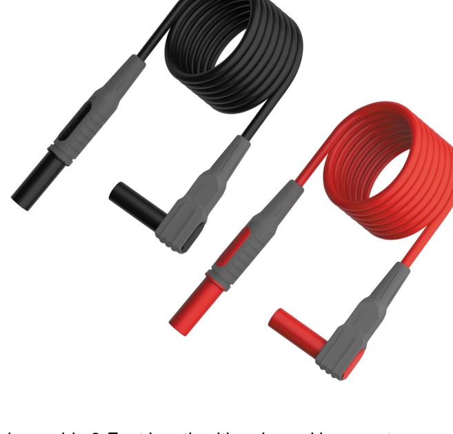
Klein Tools Replacement Right Angle Test Leads provide 3-Foot length with universal banana-type connections compatible with most clamp meters and multimeters. Features right-angle lantern input for meter connection and standard banana jack for accessories. Category III 1000V and Category IV 600V safety-rated with double insulation. Designed as an upgrade or replacement for electrical testing equipment with standard connections.
