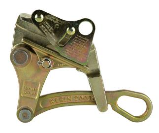
This lightweight, compact grip pulls ACSR cable from 0.16 to 0.90-Inch (0.4 to 2.3 cm) in diameter. The round jaw provides maximum contact with the cable while minimizing deformation. The hot latch closes automatically to guard against the grip accidentally disengaging from wire. This model features a locking handle to keep the jaw open while the grip is placed on the cable with a hot stick.
