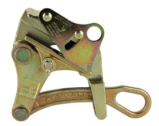
This lightweight, compact grip pulls ACSR cable from 0.16 to 0.90-Inch (2.3 to 0.4 CM) in diameter. The round jaw provides maximum contact with the cable while minimizing deformation. The hot latch closes automatically to guard against the grip accidentally disengaging from wire.
