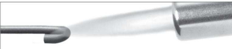
3. Heat tape to dull red and completely bend tip over 3/16" using pliers. Allow tape to fully cool.
