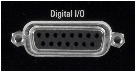
Digital I/O ports on rear panel
