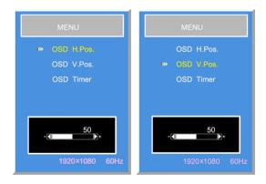
Press "enter" and "▲" or "▼" to select, and to move the OSD position in horizontal, or, vertical direction.
