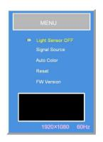
**Signal source:** Choose input source of VGA / DVI / HDMI 1 / HDMI 2 /YPbpr
