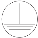
Figure Protective Conductor Terminal Symbol
