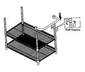
Install second batch of shelf supports onto legs to desired height of the middle shelf, and install shelf.
