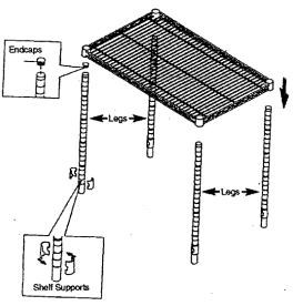
Install shelf supports onto the lowest grooves of the legs. Insert leg end caps into the top of legs. Slide legs through the corners of one shelf and fully seat onto plastic shelf suports.
