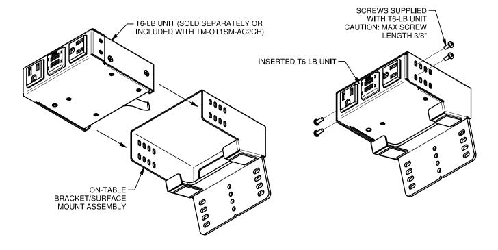
3. LOCATE AND SECURE TO TABLE/CABINET WITH SUPPLIED MOUNTING SCREWS. MAKE ELECTRICAL CONNECTIONS AS REQUIRED.
