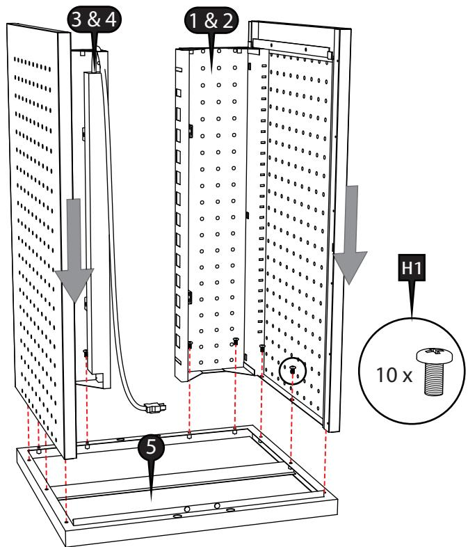
**3** Place the bottom panel (6) onto the assembly.
