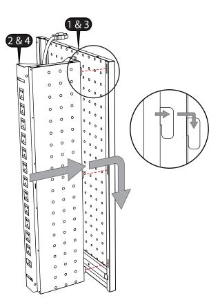
Place the bottom panel (6) onto the assembly. With a light force, secure into place.
