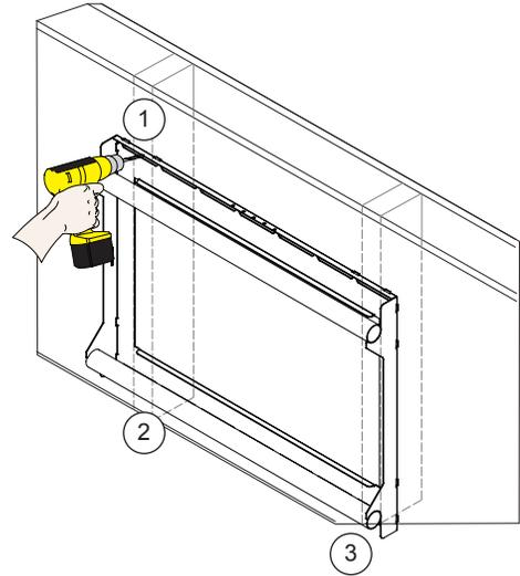
Drill a pilot hole in each of the three (3) marks with a power drill and a M6 or 1/4" drill bit.
