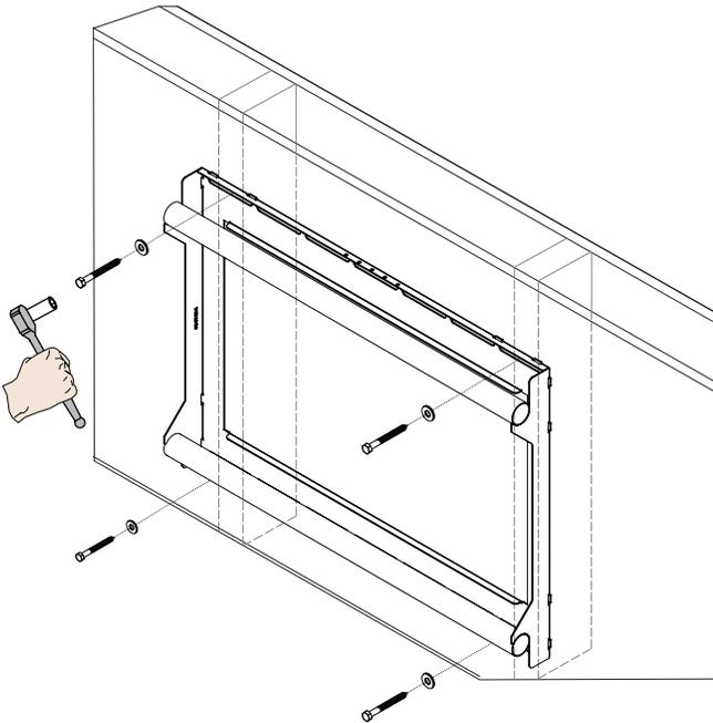
1. Insert one (1) 5/16" x 3" lag bolt and one (1) 5/16" washer into each pilot hole.
