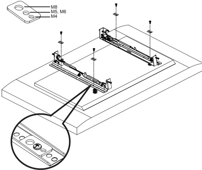
Universal Washers are designed to accommodate the various M4, M5, M6 and M8 hole sizes required by flat-panels.
