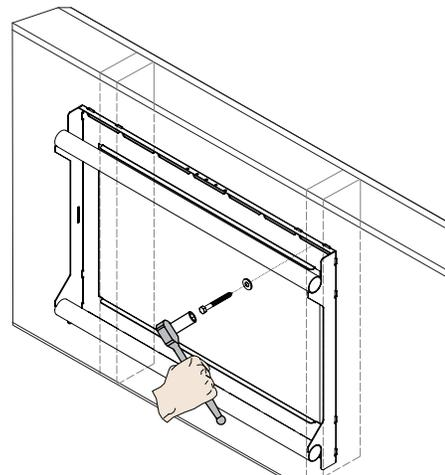
1. Place the mount against the wall and align it with the pilot hole.
