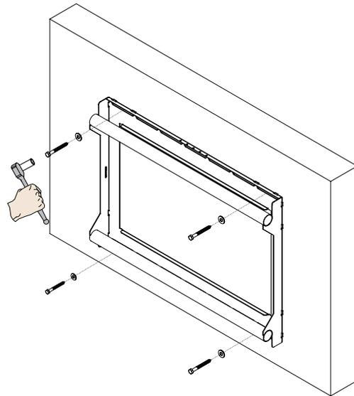
1. Insert one (1) 5/16" x 3" Lag Bolt and one (1) 5/16" washer into Finned Anchors.
