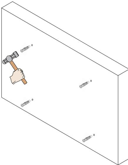
Insert the Finned anchors into each pilot holes. Lightly tap each Finned anchors into place with a hammer.
