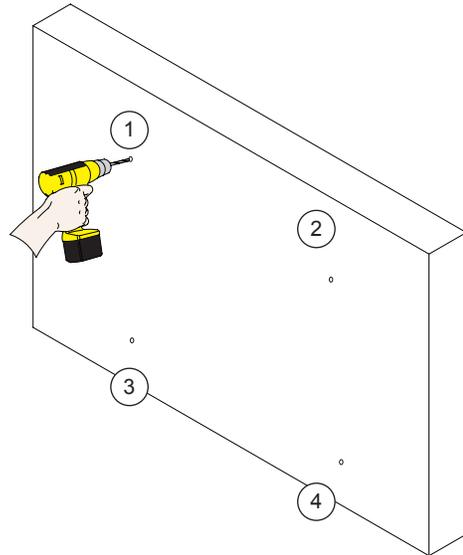
Drill a pilot hole in each of the four (4) mark areas with a 3/8" masonry drill bit.
