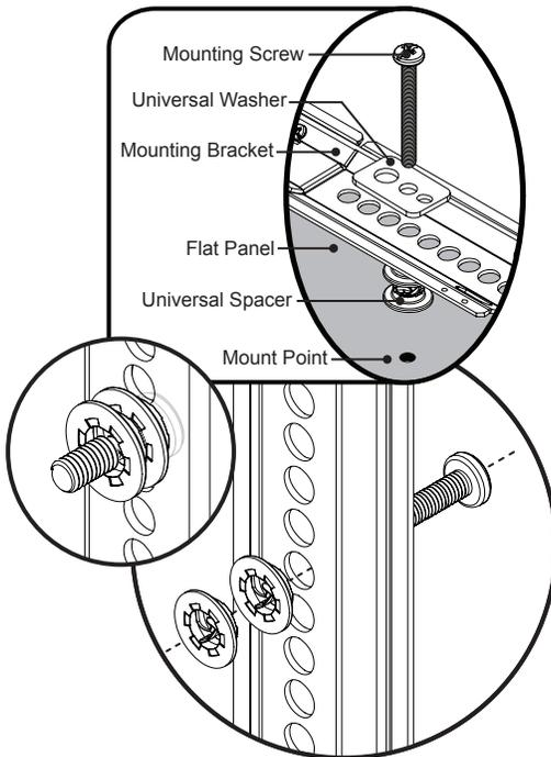
Universal Spacers allow the user to attach the mounting bracket to flat-panels which have recessed or uneven mount points. Each Universal Spacer adds 1/4" to the distance between the mounting bracket and the flat-panel.
