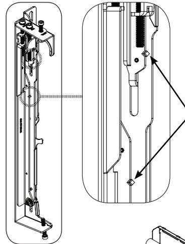
**Note:** These registers must align prior to installation. They are factory set. Check to determine proper alignment
