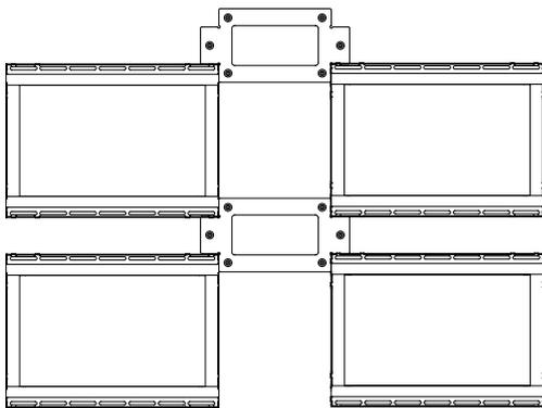
Multiple LMVF mounts can be installed using model specific spacers. Simply repeat step one when installing each of the surrounding LMVF mounts. Use one spacer for each 2x2 installation by mounting it to the wall, or utilize the same spacer as many times needed to complete an unlimited LMVF large matrix video wall.
