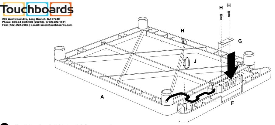
Attach electric outlet **F** to top shelf **A**, secure with L bracket **G** and cable lock **J**. Loop outlet cable **F** through cable lock **J** and the inserts on shelf **A**. Screw L bracket **G** and cable lock **J** onto top shelf **A** with screw **H** and a philips screwdriver.
