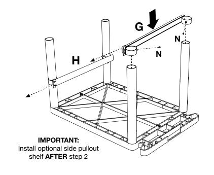
Slide and align runner **G** & **H** onto the legs
