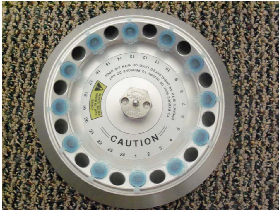
Figure 1. Loading the rotor to achieve balance
