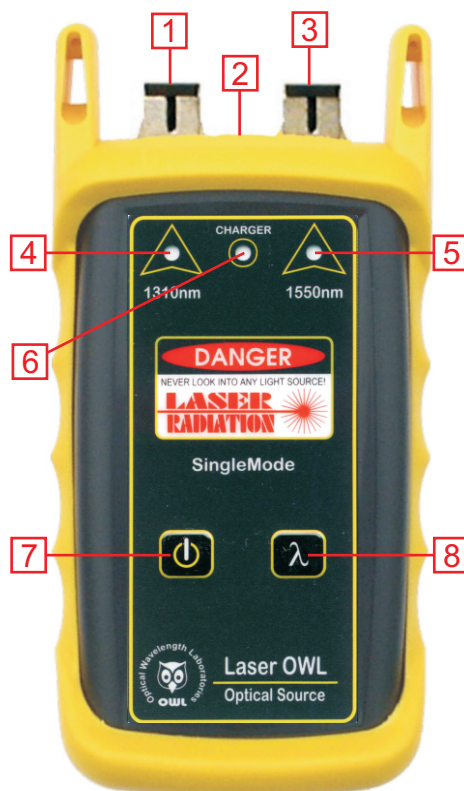
Figure 1 - Laser OWL Singlemode Laser Source
