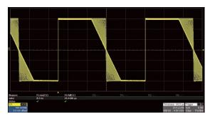
The rise/fall times can be set independently to a minimum of 1 ns (2 ns on T3AFG200) at any frequency and to a maximum of 75 s.
