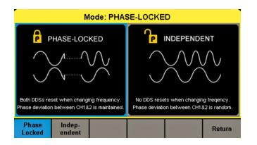
The 'Phase-Locked' mode automatically aligns the phases of each output. While 'Independent' mode permits the two output channels to be used as two independent waveform generators.
