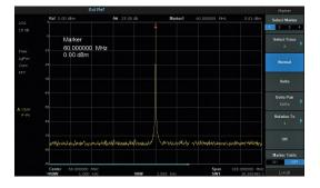
High Fidelity output with 80 dB dynamic range. Sine wave non-harmonic spurious artefacts are -60 dBc  $\leq$  350 MHz and -55 dBc > 350 MHz.
