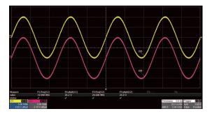
Output amplitude into a high impedance load can be as high 20 Vpp depending on frequency and waveform type.
