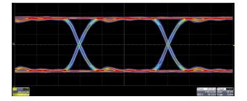
differential PRBS signals using both output channels. Easily set outputs to common logic levels such as TTL, ECL, LVCMOS, LVPECL and LVDS using built-in presets.
