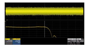
Gaussian noise with adjustable bandwidth up to 500 MHz, depending on model. Wide bandwidth Gaussian noise can be added to other waveforms to simulate real-world scenarios in which the signal contains a large degree of noise.
