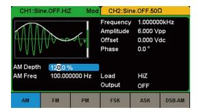
The T3AFG range of Function/Arbitrary Waveform Generators support a wide range of modulation types including AM, FM, PM, FSK, ASK, PSK, PWM and DSB-AM.
