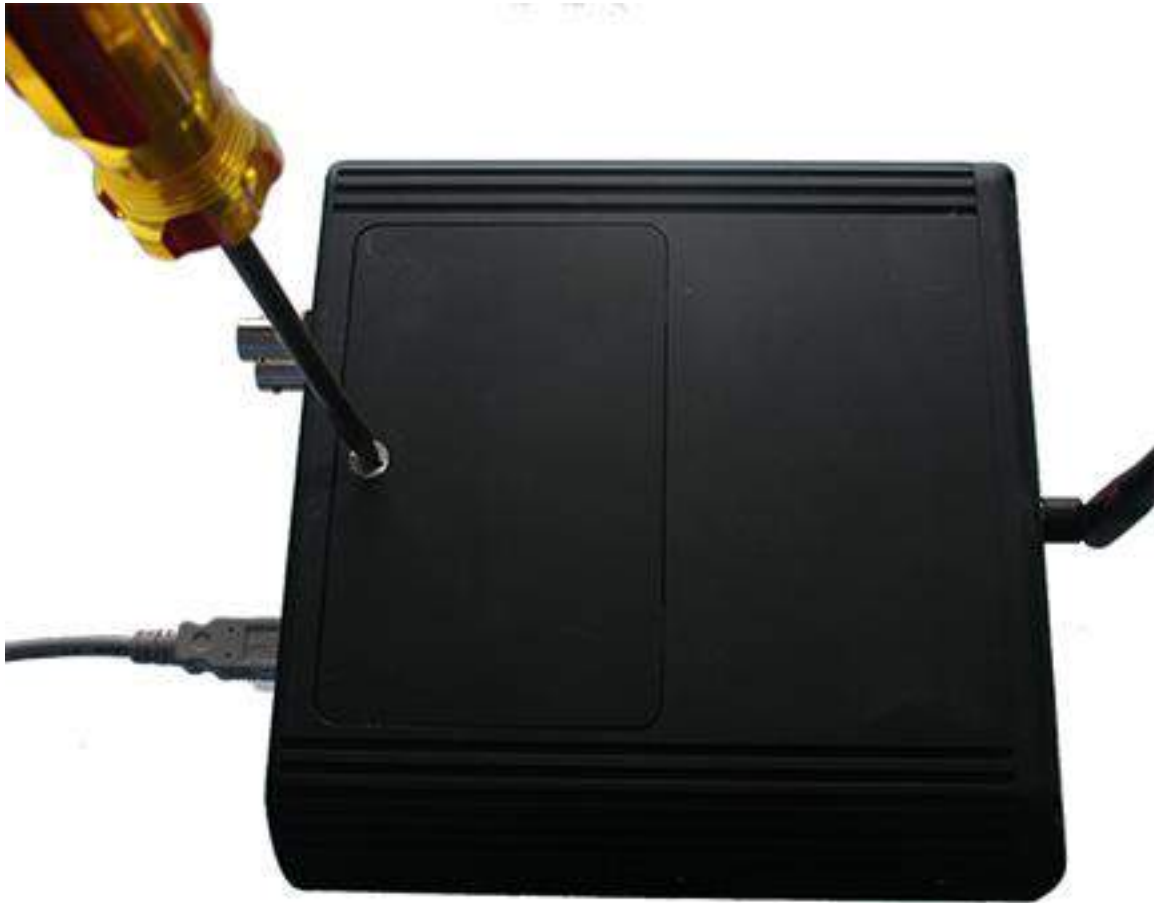
Figure 2.29 - Sodera Battery Cover, turn clockwise to secure
