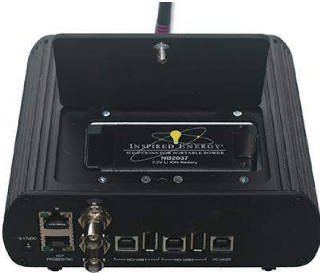
Figure 2.24 - Soderas Battery Compartment with Cover Opened
