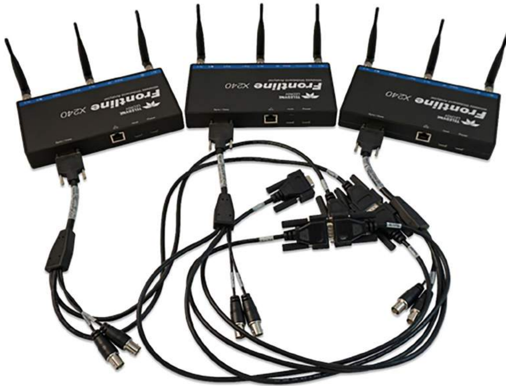
Figure 2.20 - Three X240 Units connected with CATC Sync Cable Kits
