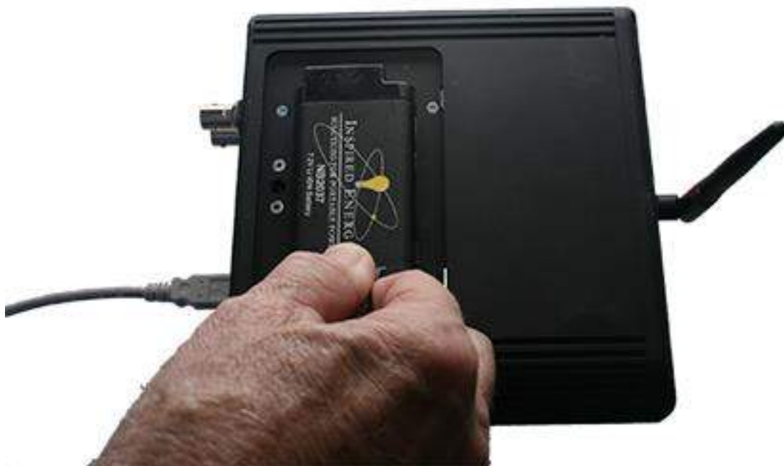
Figure 2.25 - Sodera Battery Removal Using the Tab
