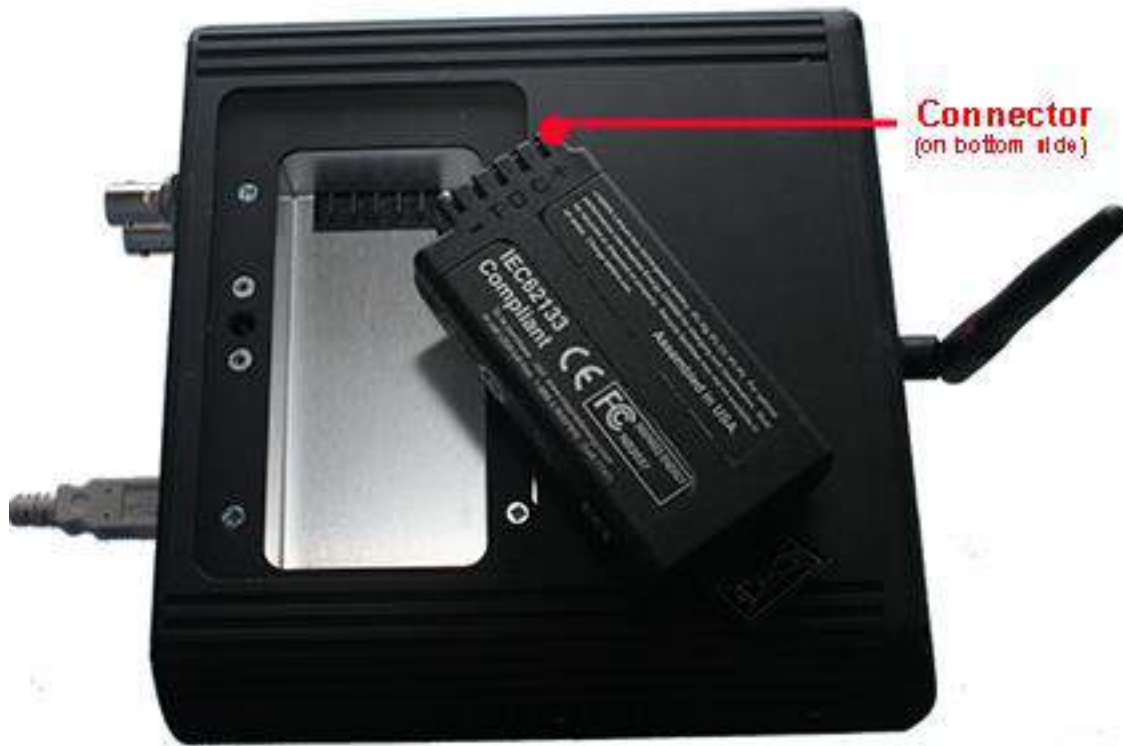
Figure 2.26 - Sodera Battery Connectors, bottom side shown.
