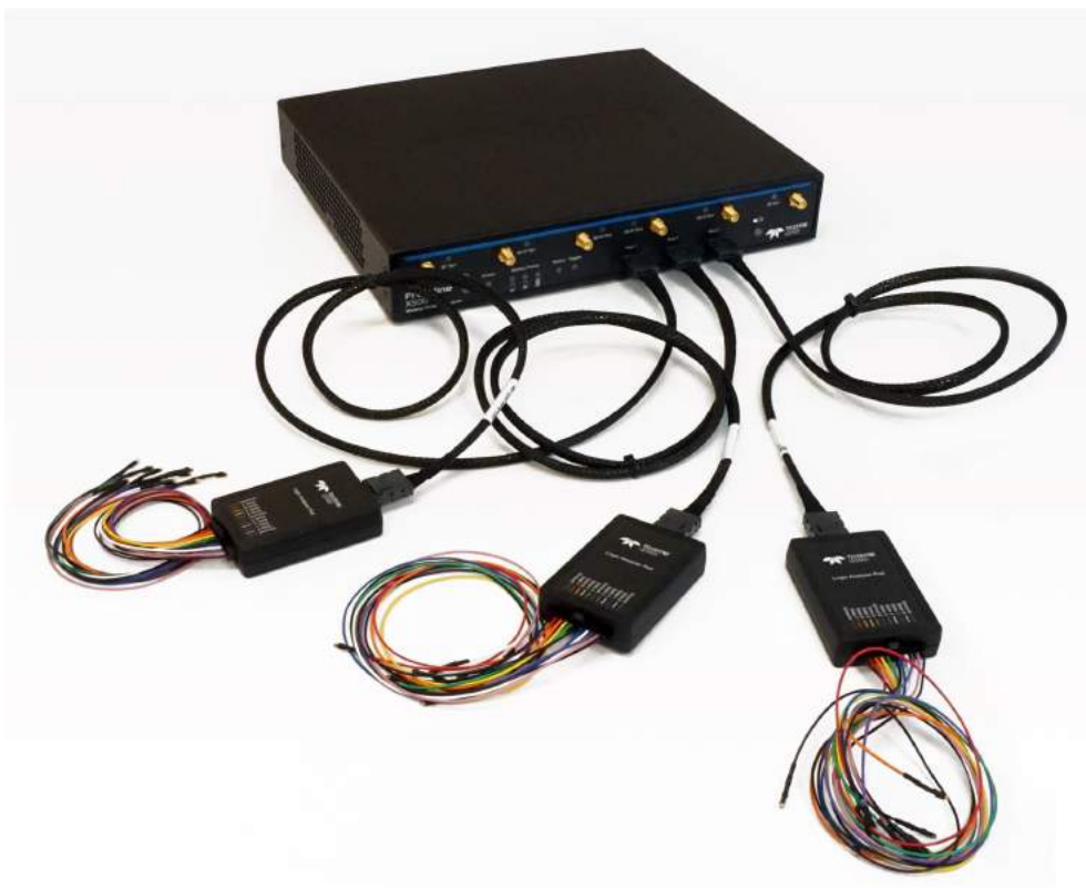
Figure 2.4 - X500 Logic Analyzer Pods Installed on X500
