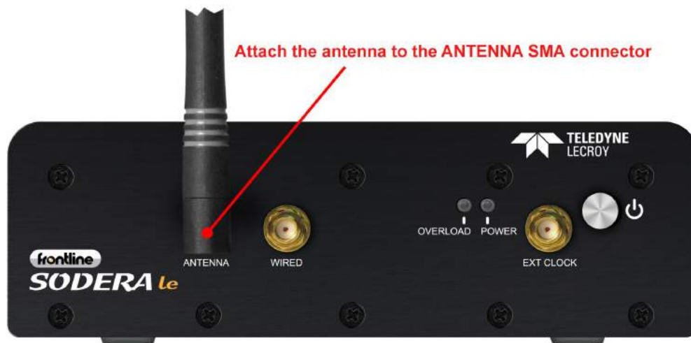
Figure 2.37 - Antenna Attachment Point
