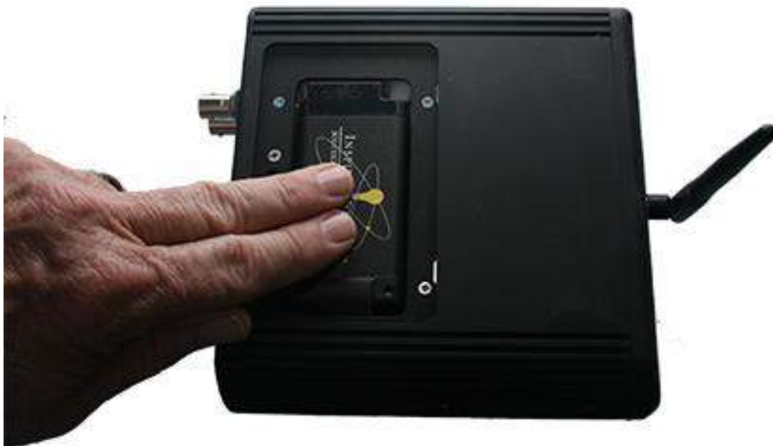
Figure 2.27 - Sodera Battery: Press to Make Contact
