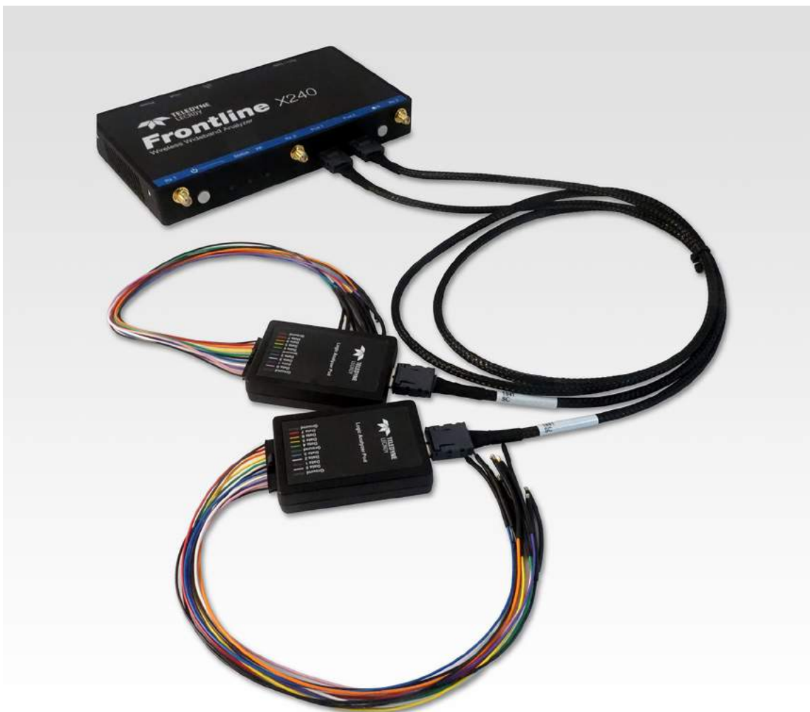
Figure 2.12 - X240 Logic Analyzer Pods Installed on X240
