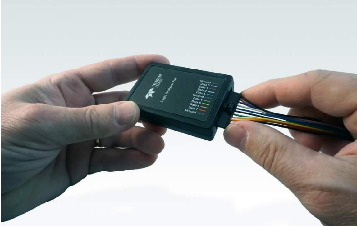
Figure 2.14 - Installing the Flying Lead Assembly on the X240 Logic Analyzer Pod
