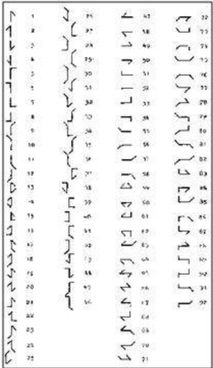
Figure 11 - Chappe's Telegraph Code
