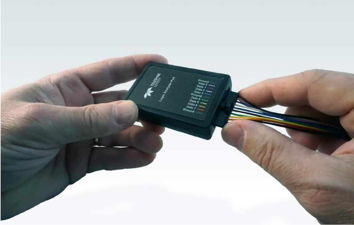
Figure 2.6 - Installing the Flying Lead Assembly on the X500 Logic Analyzer Pod
