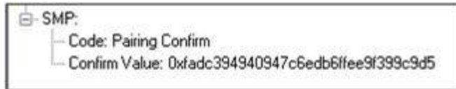
Figure 13 - Initiator Pairing Confirm Example (Wireless Protocol Suite software Main windows, Sodera, Sodera LE Low Energy capture)
