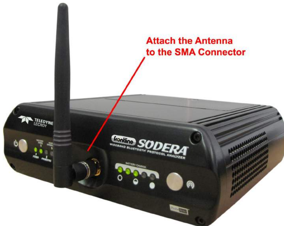
Figure 2.23 - Antenna Attachment Point
