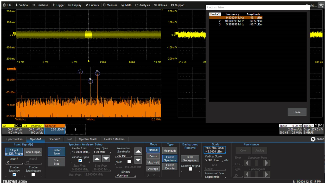
Spectrum of input signal prior to background removal. A third peak belonging to the signal is identified.
