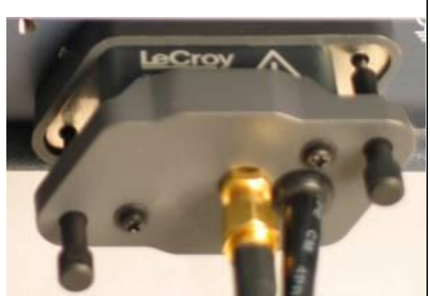
Connection of the TF-DSQ Fixture to the Oscilloscope Input
