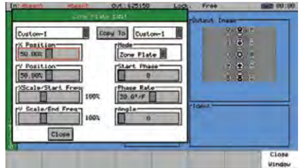
The 'moving zoneplate' configuration window. Multiple saves of parameters can be made.
