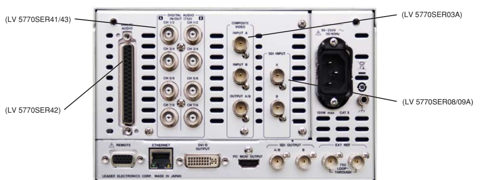
Example of an LV 5770A with an LV 5770SER03A, LV 5770SER09A, LV 5770SER41, and LV 5770SER42 installed. (Connect Pic Moni Output to a monitor that supports HDMI input.)
